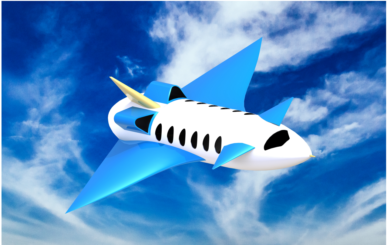
Figure 18: Conceptual rendition of the Goldeneye AB1 supersonic business jet in supersonic cruise wing configuration, with its canard, vertical stabilizer, and engine nacelles on display.
